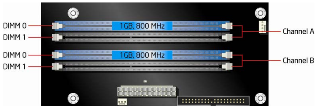
Figure 17. Dual Channel Memory Configuration with Two DIMMs
